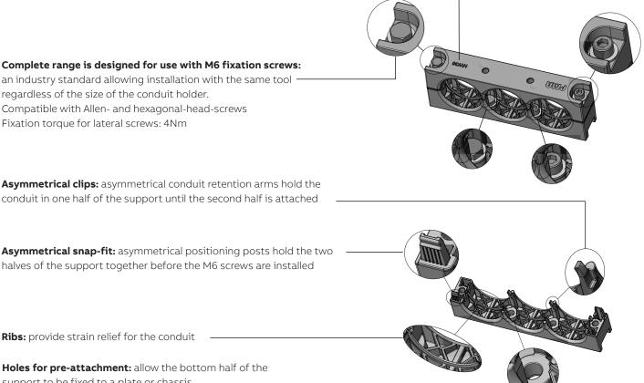
Holes for pre-attachment: allow the bottom half of the support to be fixed to a plate or chassis For mounting on C-rails: Fixation torque for pre-attachment to be < 2Nm
